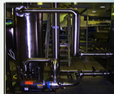
OOO «Nestle Water Coolers Service» – a system of water ozonization with capacity of the ozone 150 g/h
