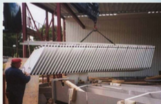
The lower part of the clarifier with the thin-layer modules
